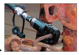
Steel rope is easily cut with the smooth guillotine action of an Enerpac cutterhead.
